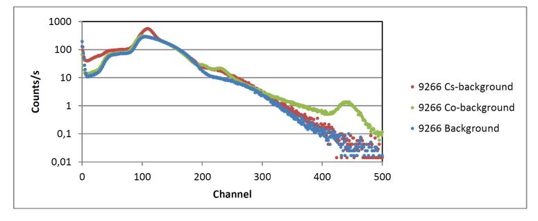
This figure shows the results obtained with PMT 9266 for 3 different scenarios: without any source, with 137Cs next to it and with 60Co. Clearly visible is the contribution of the 137Cs peak, as well as the two peaks from 60Co. For the latter one the sum peak around channel 450 can be seen clearly as well.
